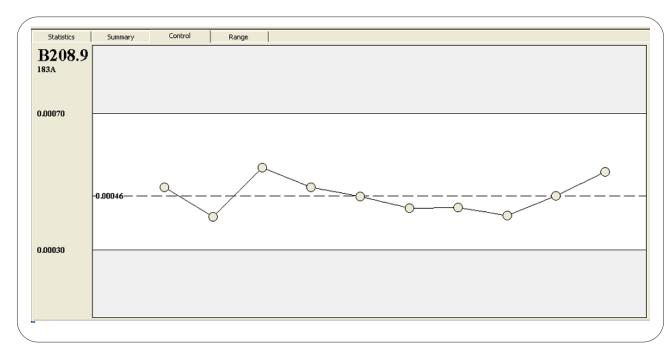
Screen shot demonstrating the control charting ability of the GDS500A. Upper and lower limits were automatically calculated by the software at  $2\sigma$ .
